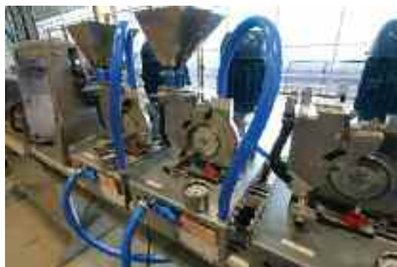
The seeders are unique, featuring vertical spinning disks that drop the seeds into the gutters passing beneath.
