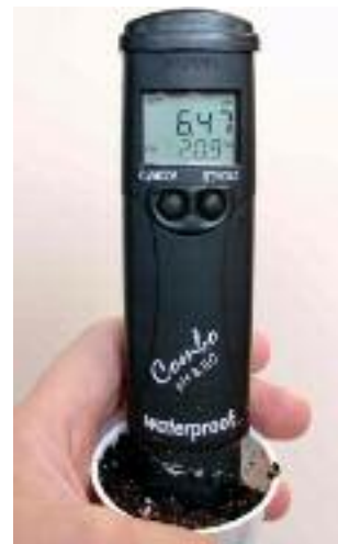
A combination EC and pH meter is used to measure these parameters of a growing medium sample.
